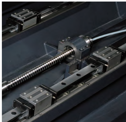
High rigid linear roller guides are used for all axes of X, Y and Z.
