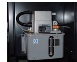
Automatic lubrication unit for magazine and ATC part [Opt]
