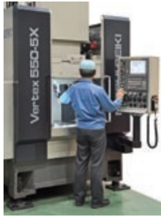
Accessing the table surface is very easy and comfortable for the operator because of the stationary table design.
